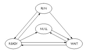
Figure 1 is an example of task states and task-state transitions. This diagram is representative of most kernels. NULL means that the task has not been created yet or has been deleted. WAIT means it is waiting for an event. READY means it is ready to run. RUN means it is actually running. In a single-processor system, only one task at a time can be in the RUN state. Most of the time, this task will be the highest-priority task that is ready to run.
